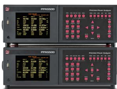
PPA5500 units in Master/Slave mode, synchronised for 4-6 Phase measurements
