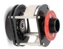
The AS613 series is a rugged free end with support for the pneumatic pipe-work coming out of the back of the assembly. It features a locking ring with integral safety lock which prevents accidential operation and indicate that the Circlex plates are locked together correctly.
