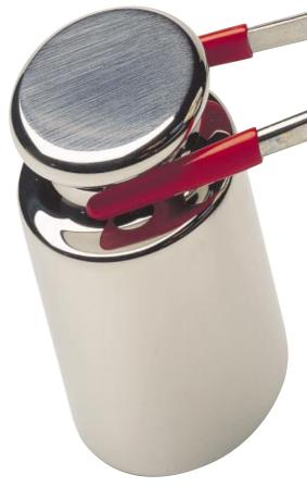
plastic tipped tweezers can become contaminated with dirt, which is then transferred on to weights which are being handled.
