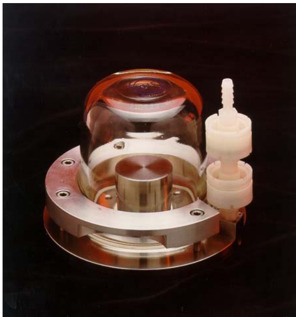
Figure 1: The UK national standard kilogram
