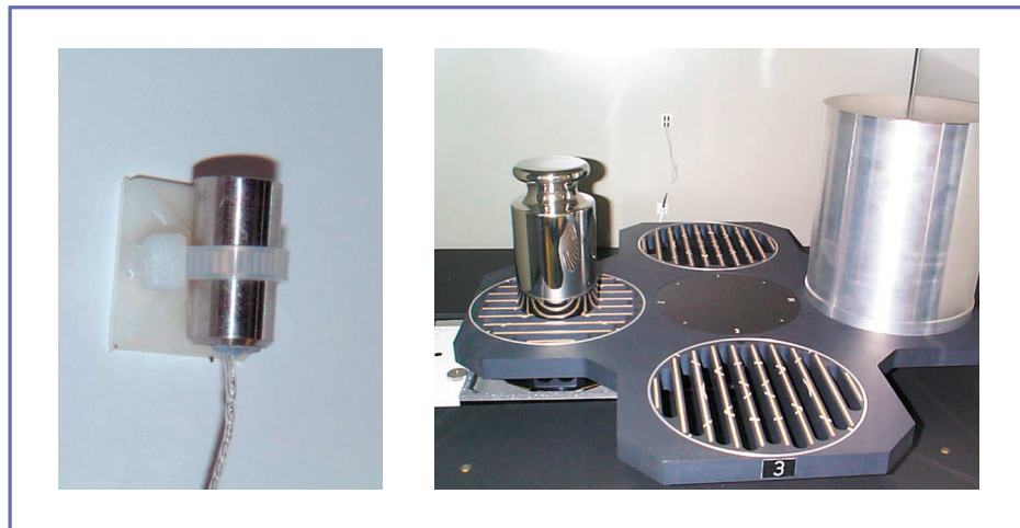
Figure 1: Thermistor probe and its siting in a balance enclosure
