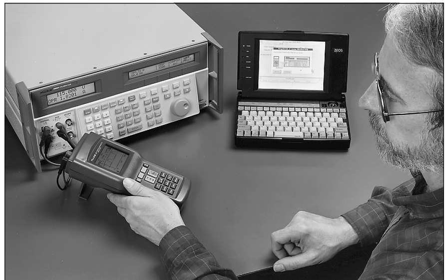
The 5500A Multi-Product Calibrator is specified at a 99% confidence level, as are all Fluke calibrators and standards.
