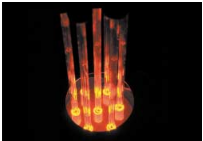
A batch of Hart SPRTs being annealed in a specially constructed, non-contaminating furnace.
