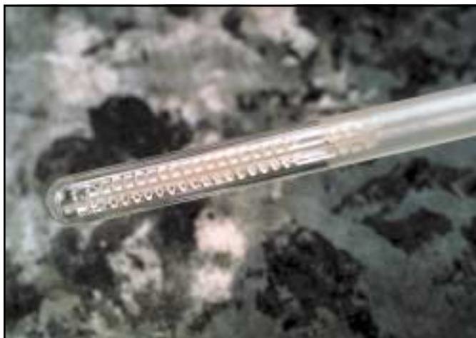
A close-up of a 25-ohm spiral-wound helix SPRT element.
