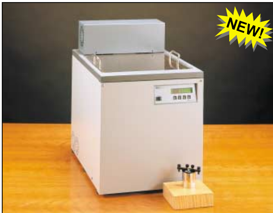
Peltier-Cooled Resistor Bath Model 7108 Stability of ±0.002°C, uniformity of ±0.005°C Peltier cooling provides quiet operation and lower heat dissipation
