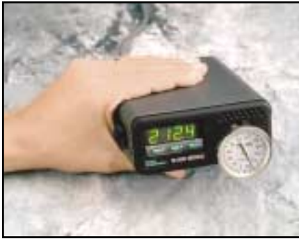
Handheld block calibrators have made industrial calibration more portable.
