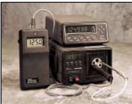
Calibrations using dry-wells can be improved by using an external reference such as the 1502 Tweener Thermometer.
