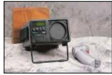
Watchfor the release of Hart's newest IR calibrator. Coming in 2001, the Model 9132 covers temperatures to 500°C with a large, 2¼-inch blackbody target.
