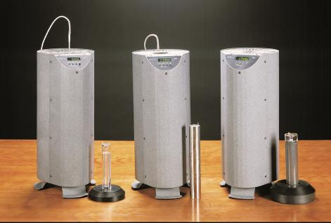
In addition to the 9230 Gallium Maintenance System, Hart's 9210 Triple Point of Water Maintenance System and 9260 Mini Fixed-Point Furnace simplify the use of ITS-90 fixed-point cells. Each offers built-in software for automated realizations and provides uncertainties similar to larger traditional systems.
