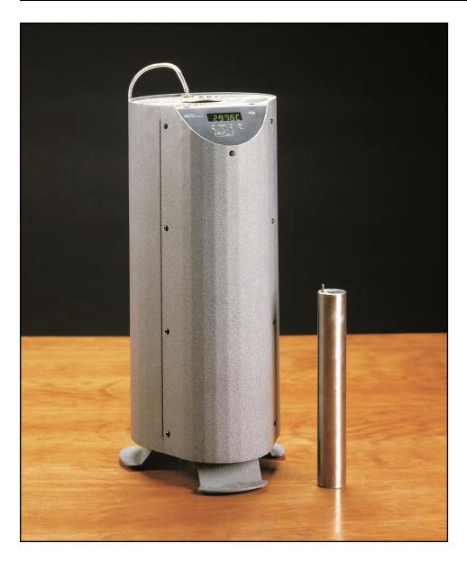
The gallium melting point (29.7646°C) is a critical temperature. Thermometers used in life science, environmental monitoring, and many other applications depend on it for accurate calibrations. Lab standards rely on it as an ITS-90 check standard and as a means of measuring drift between calibrations. Hart Scientific now makes it easy to use.
