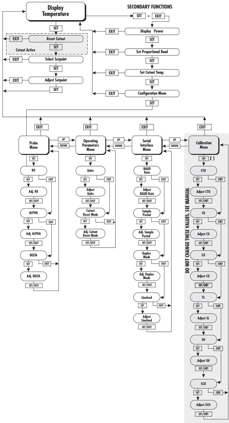
Figure 3 Controller Operation Flowchart
