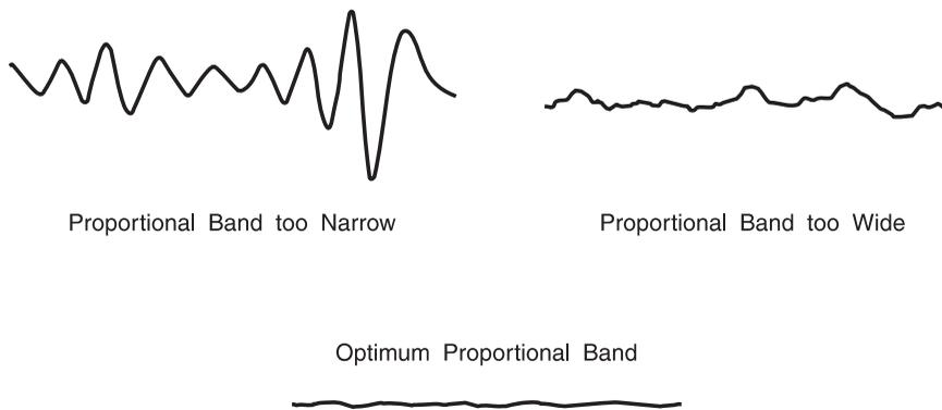
**Figure 4** Strip chart recordings showing various proportional band settings
