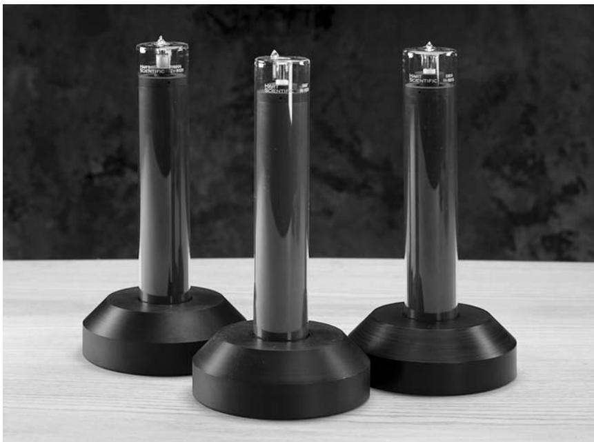
**Figure 1** *The metal freezing point cell.*
