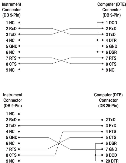
**Figure 13.** Serial Cable Wiring.
