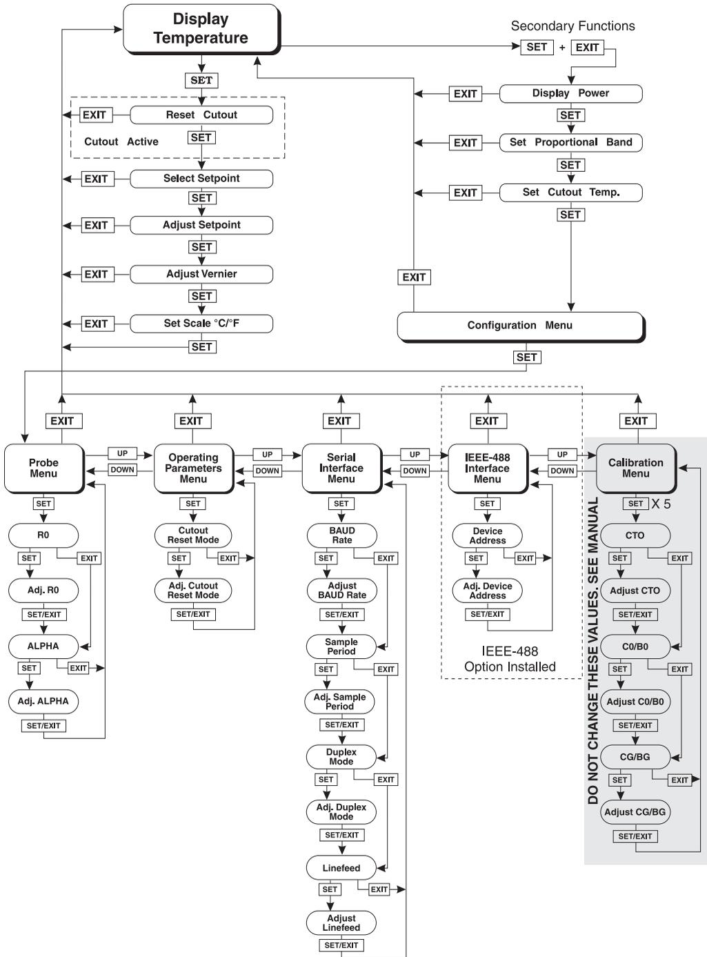
Figure 9. Controller Operation Flowchart.
