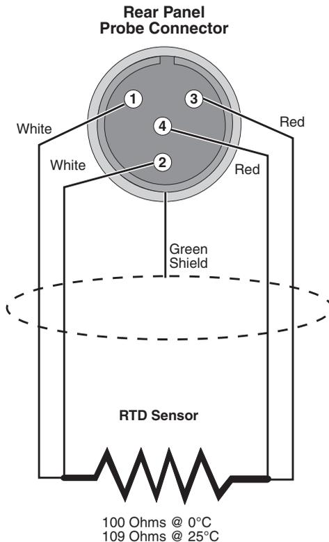
**Figure 12.** Control Probe Connections.
