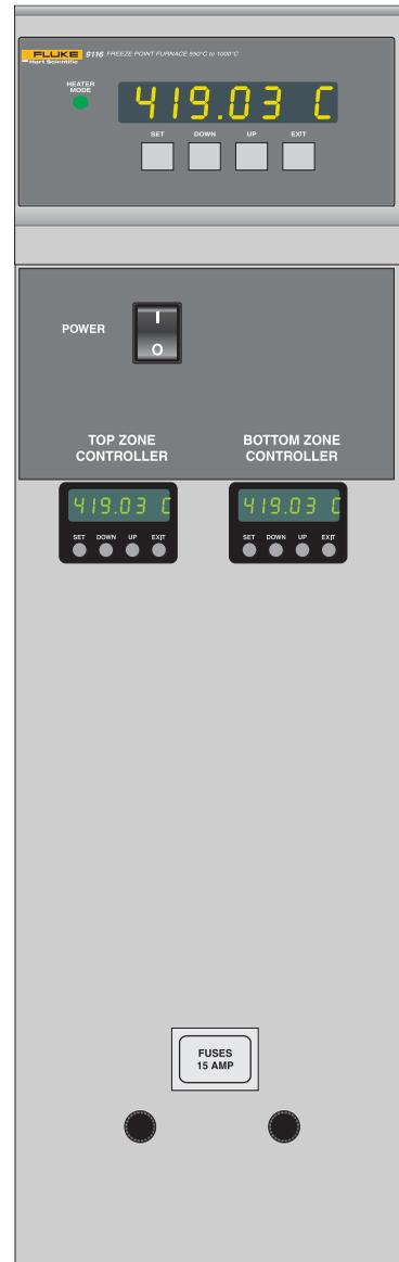
**Figure 5** Front Control Panel (cover door removed)
