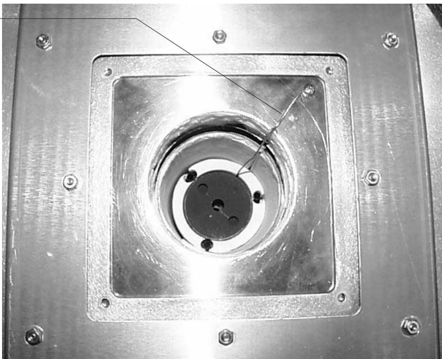
**Figure 3** Attachment of Heater Ground Wire to Furnace Chassis
