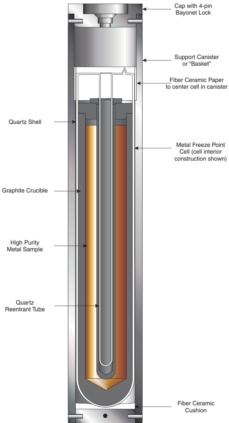
Figure 10 Metal Freeze Point Cell Installed in Canister
