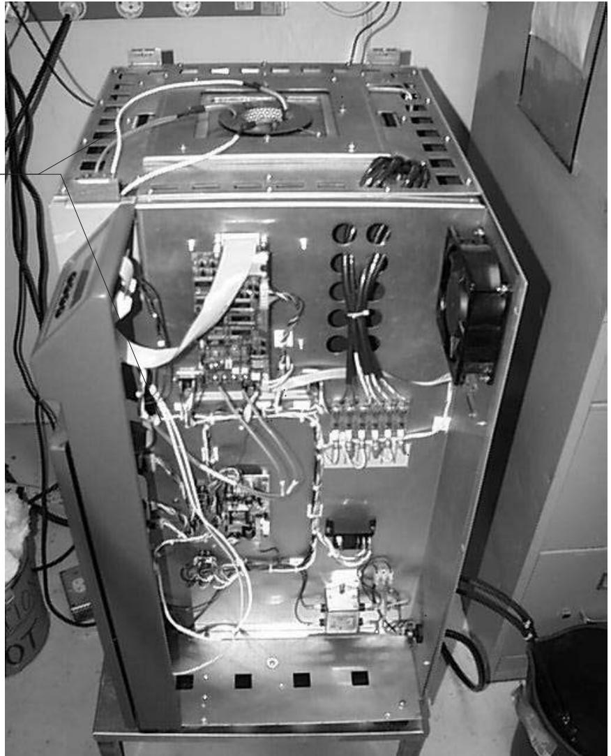
**Figure 4** *Thermocouple Wire Routing*
