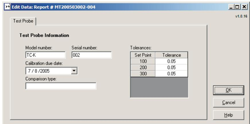
**Figure 6** Edit Data dialog – Test Probe tab for thermocouple probes
