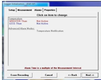
The loggers support two different methods of measuring the time for an alarm condition. The default method is “Cumulative Time”. The total time beyond the limit is counted. The alarm limits may be exceeded only once or several times as the total time is added together. The second method is called “Continuous Interval”. The alarm will activate only when the alarm limit has exceed the full time specified. If the temperature returns to the acceptable range the time count will be reset.
