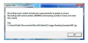
The EZ Logger must contain at least 2 measurements. If you try to read the EZ Logger before it has captured 2 data points you will see this warning. If this window appears click **OK** and wait for more time to pass.
