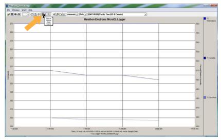
The **Change Line Style Icon** is used to change the color and width of the plot lines.
