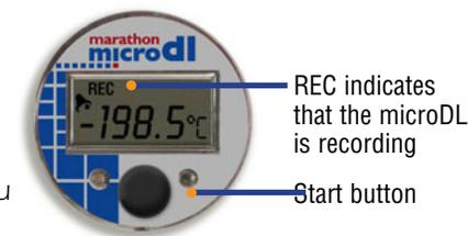
The microDL can now be placed where you want to record the temperature.
