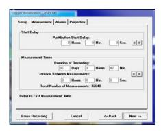
Conversely, setting the "Interval Between Measurements", will automatically calculate the "Duration of Recording".
