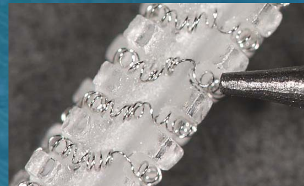
This sensor was damaged by vibration. Notice shorting of coils.
