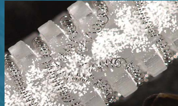
This sensor was damaged by shock during shipping and handling
