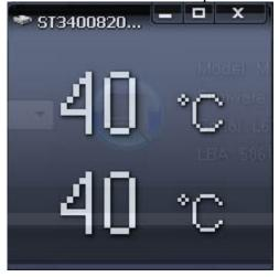
For SCSI drives the information window shows two values. The second value is shown on the Task bar and represents current temperature.
