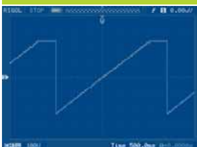
DC Voltage ramp
