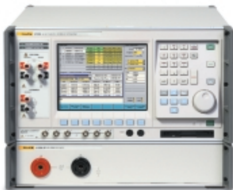
6100A/E/80A Electrical Power Standard
