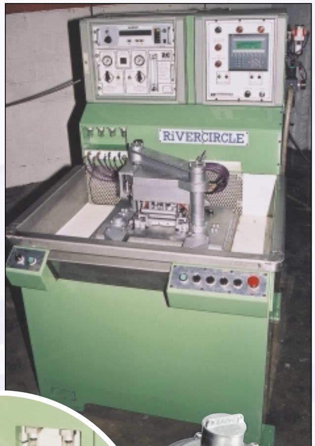
Manifold Dry Leak test Rig with heavy duty pneumatic sealing fixture
