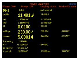
Where users wish to see measured functions at higher resolution, any selected measurements can be viewed with a 6 digit display. Here, we see 6 digit presentation of items selected in the first screen.
