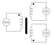
Select 'Vector Voltmeter' mode and using the SETUP menu select 'LVDT ratio' as the parameter. Enter the electrical stroke of the LVDT in meters as the scale factor (if required). The magnitudes of the two inputs are computed by DFT analysis at the fundamental frequency. The displacement is computed as:
