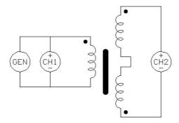
Select 'Vector Voltmeter' mode, and using the SETUP menu select 'LVDT diff' as the parameter. Enter the electrical stroke of the LVDT in meters as the scale factor (if required). The in-phase component of the secondary is computed by DFT analysis at the fundamental frequency. The displacement is computed as:
