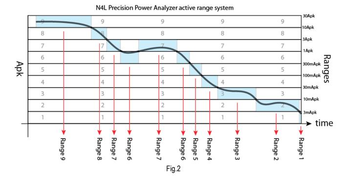
Fig.2 illustrates how an active ranging system reacts to a changing input signal, dynamically adjusting its range as the input signal changes in magnitude.
