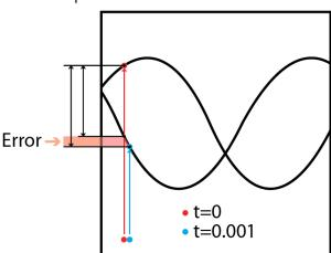
Fig.3 – Multiplexed phase-phase Vrms measurements cause errors
