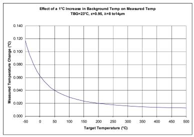
Figure 2. Effect of a 1°C Change in Background Temperature
