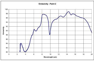
Figure 3. Emissivity of a Typical Paint
