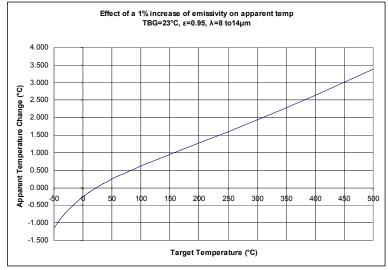
Figure 1. Effect of a 1% Change in Emissivity
